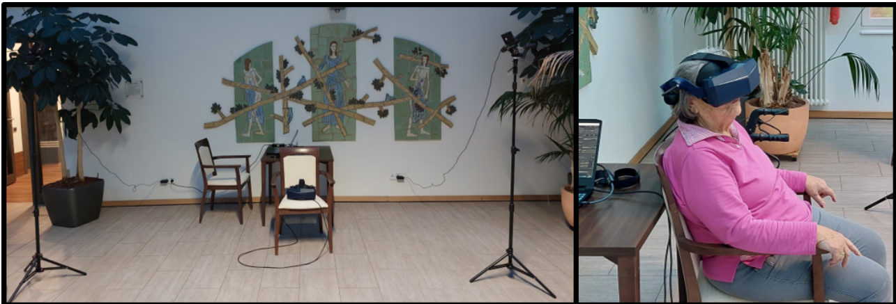
Figure 2. Virtual reality setup. Chair between 2 SteamVR Base Stations 2.0 with Pimax Vision 5k super (top). Participant with head-mounted display (HMD) and virtual park environment (bottom).
