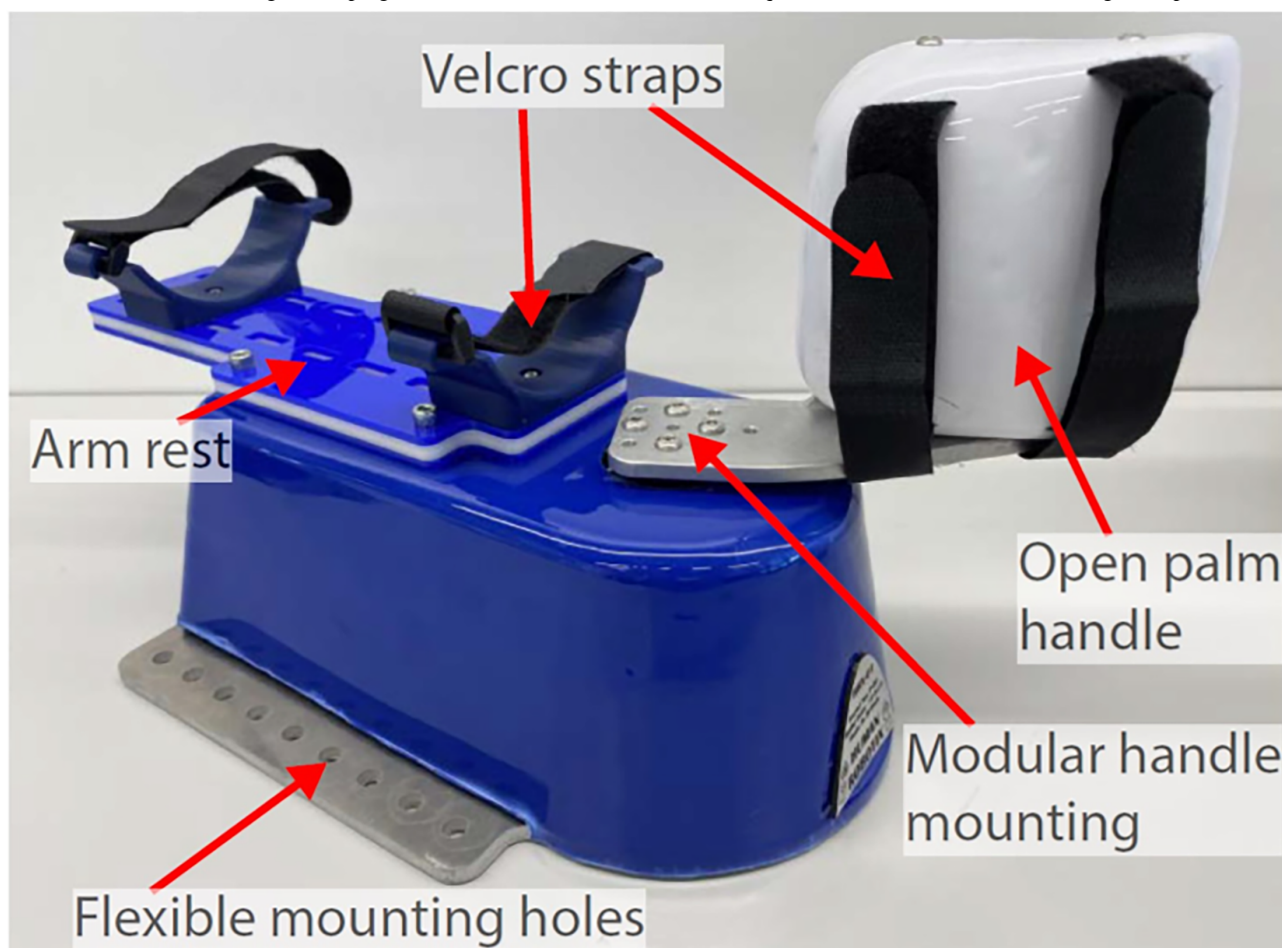
Figure 2. HRX-1 robot that can generate programmable wrist flexion and extension torques for assistance or resistance during the experimental study.
